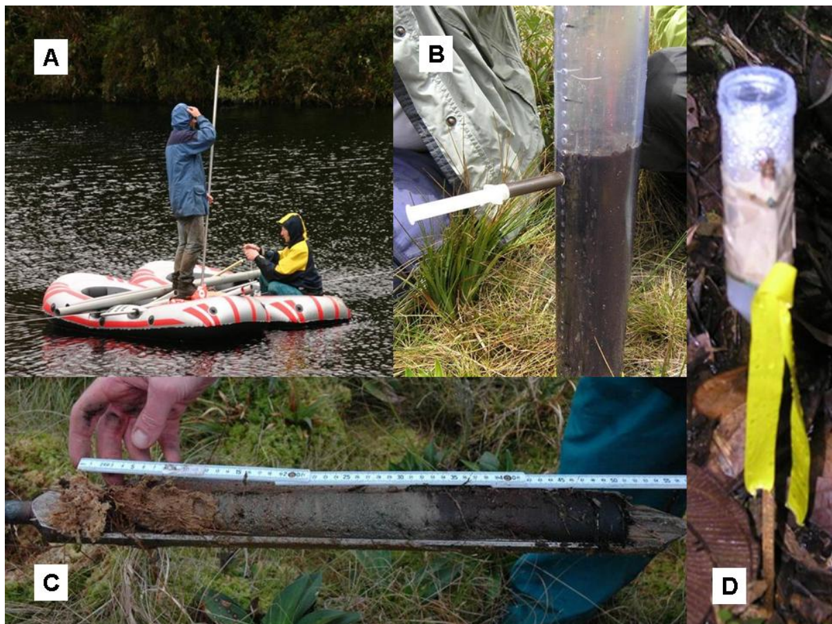
Figure 1.3: Field work methods: Lake sediments were explored with a Livingstone piston-corer (A) and/or the Kajak-Corer (B). The Russian corer (C) was used for peat bog deposits. Pollen traps (D) were installed to collect recent pollen rain.
